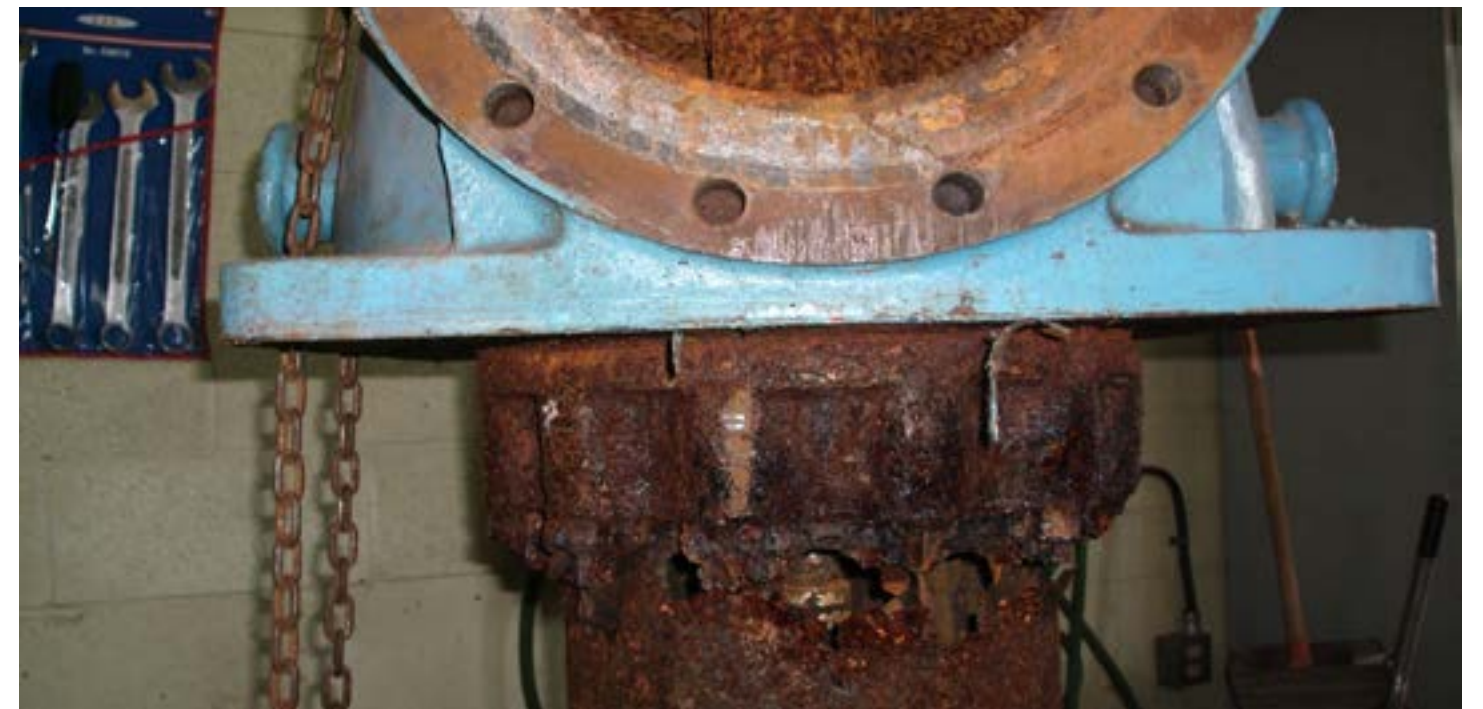
Partially corroded vertical turbine pump column attached to the discharge head. Pump still functioned at a lower efficiency of course!
